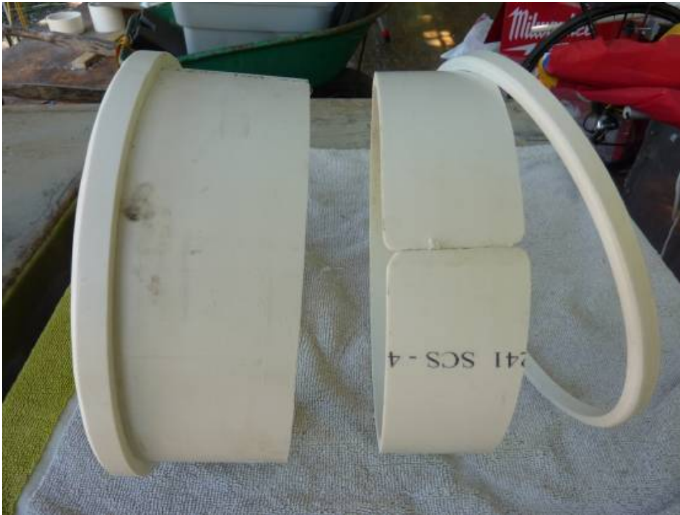
Left: PVC portal with retainer ring attached, Middle: stabilizer piece, Right: loose retainer ring
