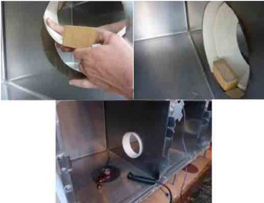
Top left: Placing the stabilizer piece and wooden block to open. Top right: stabilizer in place and portal being slid into stabilizer. Bottom: portal in place.
